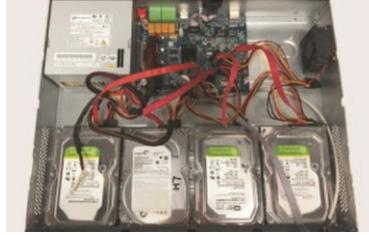
**Tips:** Please check the inside structure of the device and make sure the cables connected well before installing the cover back. Please format the HDD before using.
