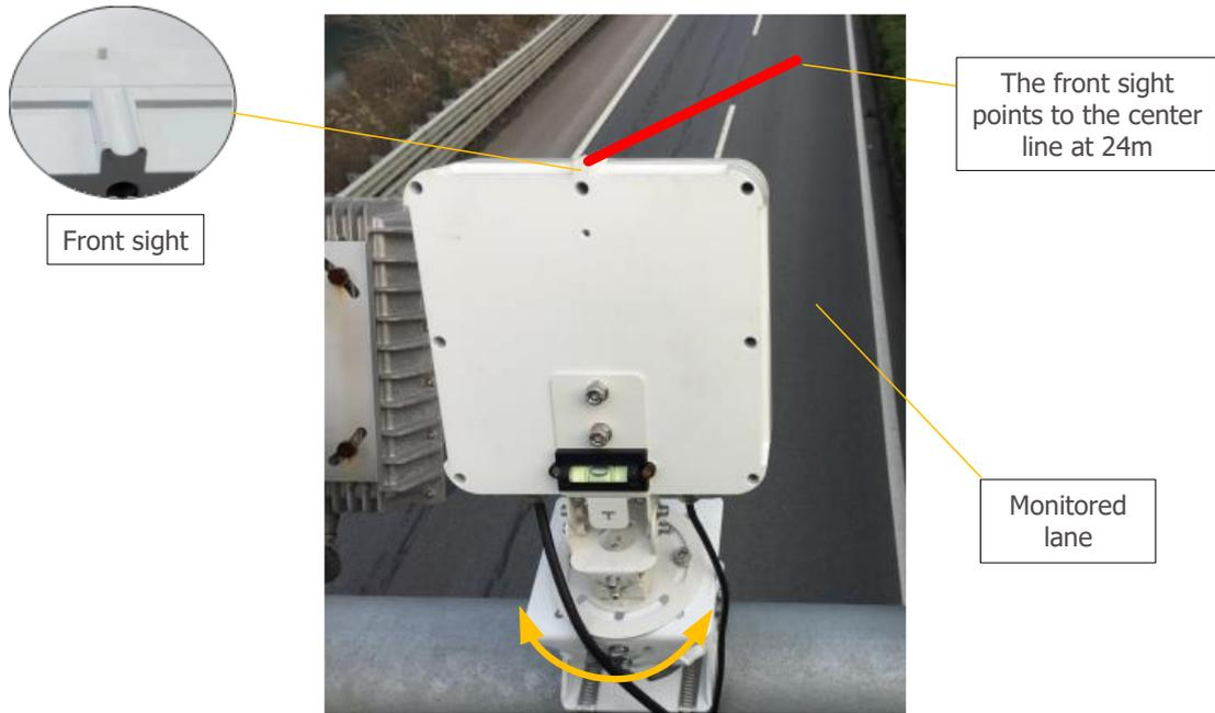
Figure 10 – Horizontal rotation diagram
