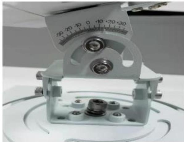
*Figure 5 – Pitch angle recording*
