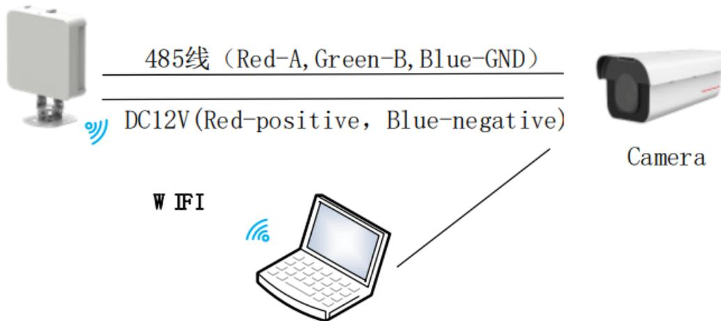
Figure 7 – Schematic diagram of radar connection
