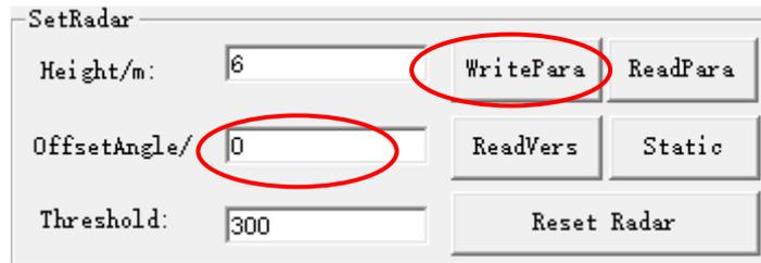
Figure 13 - Installation height and deflection angle settings
