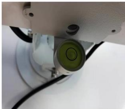
Figure 3 - Schematic diagram of horizontal state adjustment
