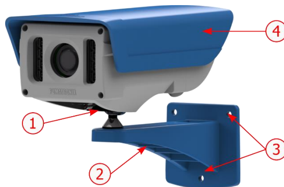
Figure 4 - Fixing the 450+ Bracket: 1) 450+ device tilt adjustment; 2) 450+ Bracket; 3) Fixing points, using 3/16" screws; 4) Sliding Flap, adjusted in the framing
