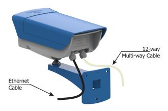
Risk of Oxidation: The electrical and signal connections made in the ITSCAM 450+ bundle and the data network cable must be protected in a terminal box or similar structure to prevent oxidation of the connections and unwanted infiltration of liquids into the bundle.
