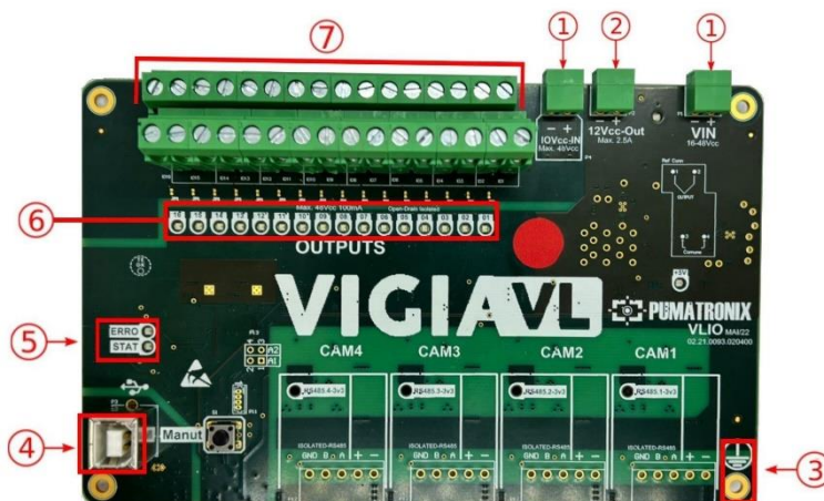
Figure 7 - VLIO Board Interfaces: 1) Power Inputs; 2) Output connection for Firefly (ULP) power; 3) Board grounding (must be connected to the GND of the Installation); 4) USB data connection; 5) ERROR and STAT LEDs; 6) LEDs indicating Output signals; 7) Signal outputs to the Traffic Controller
