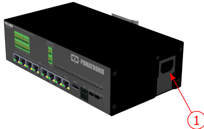
Figure 9 - Power connector (AC cable)
