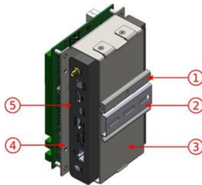
Figure 20– 1) DIN Rail Support; 2) DIN Rail 75mm; 3) Bottom Support; 4) Top Support; 5) ULP
