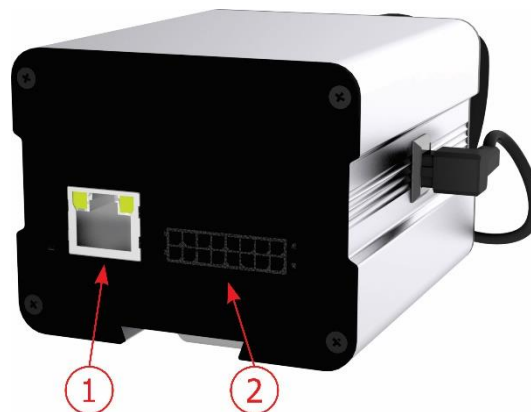
Figure 7 - Interfaces available on the device: 1) Ethernet; 2) Microfit 16-way (power connector, IOs, RS-232)
