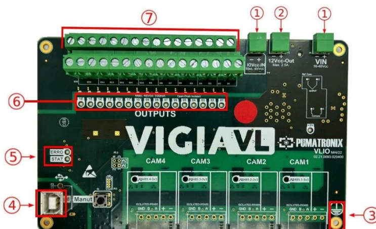
Figure 7 - VLIO Board Interfaces: 1) Power Inputs; 2) Output connection for Firefly (ULP) power; 3) Board grounding (must be connected to the GND of the Installation); 4) USB data connection; 5) ERROR and STAT LEDs; 6) LEDs indicating Output signals; 7) Signal outputs to the Traffic Controller
