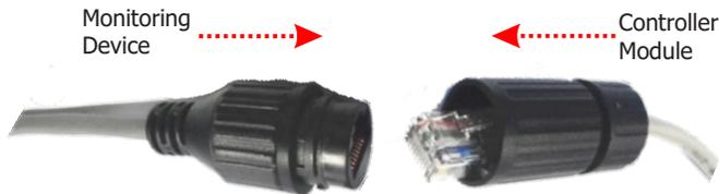
**Step 7:** Close the Coupling Connector, connecting to the monitoring device:
