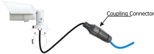
**Step 8:** Position the Coupling Connector assembled with Ethernet cable on the Pole Bracket.
