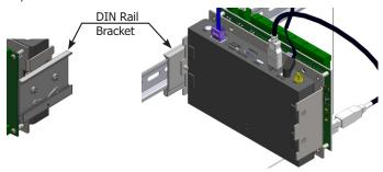
**Step 23:** Snap the module onto the panel rail.
