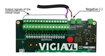
**Step 29:** Fill in the Installation Mapping with the data for the OUTPUTS terminal blocks used for connection, identified as I/O Ports in the software interface.
