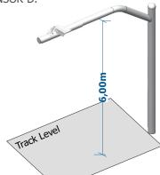
To use the VL-SENSOR-D in the vertical position, additionally install the VIGIA-VL Stand. However, installation on the side of the road can cause occlusion of vehicles traveling in the far lane.
