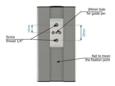
**22.** Reassemble the fixing mechanism following the sequence indicated in the image, if it detaches from the ITSCAM 450 housing:
