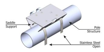
**Step 9:** Align the surface of the post holder with the plane of the via.
