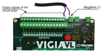
**Step 27:** Fill in the Installation Mapping with the data for the OUTPUTS terminal blocks used for connection, identified as I/O Ports in the software interface.
