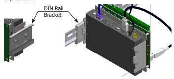
**Step 21:** Snap the module onto the panel rail.
