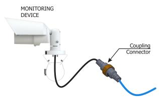
Step 6: Position the Mating Connector assembled with Ethernet cable on the Pole Bracket.
