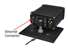
**2.** Use cable with RJ-45 connector following the pinout of the TIA-568A standard:
