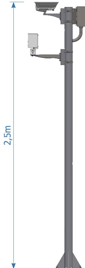
*Figure 11 - Panoramic Post with ITSCAM VIGIA+, ITSLUX (optional) and Terminal Box attached*
