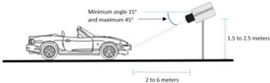
Figure 12 – ITSCAM installation for toll, parking lot and similar situations (side view)
