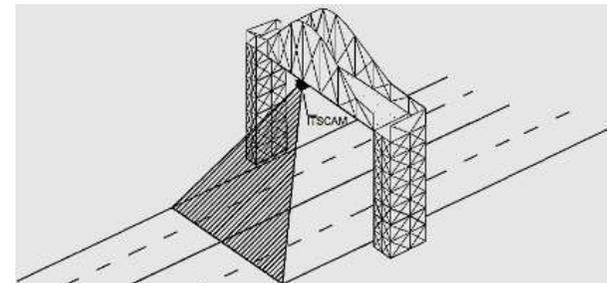
Figure 46 – ITSCAM installation maximizing Vehicle Counter results
