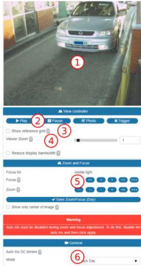
Figure 40 – Zoom and Focus Settings at ITSCAM Web interface
