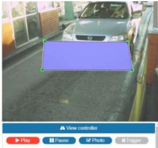
Figure 44 – ITSCAM Web interface with a Region of Interest (ROI) set. The OCR algorithm will search for plates placed in the ROI.
