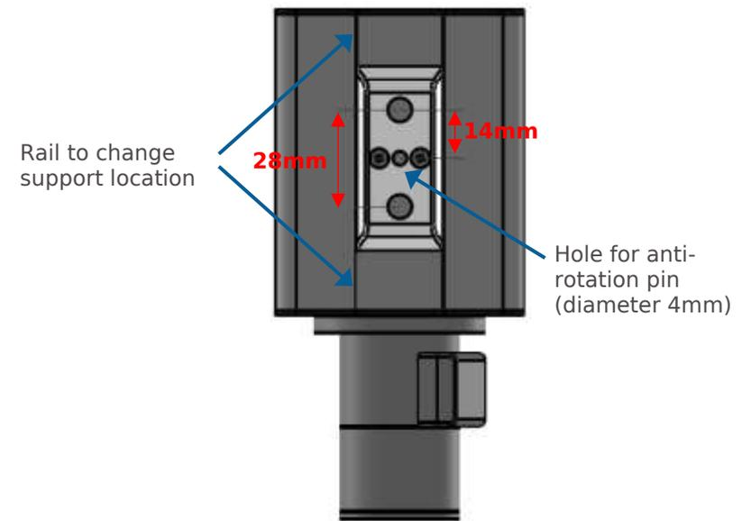
Figure 16 – Bracket specifications
