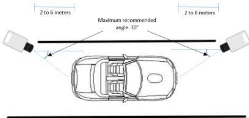
Figure 13 – ITSCAM installation for toll, parking lot and similar situations (top view)
