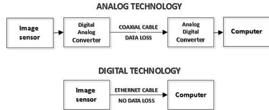
Figure 1 – Comparison of digital and analog image conversion steps
