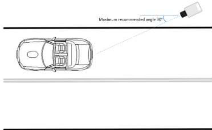
Figure 15 – ITSCAM installation for traffic control (top view)
