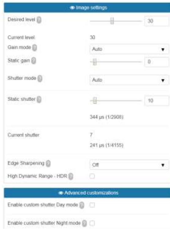
Figure 37 – Image Settings at ITSCAM Web interface
