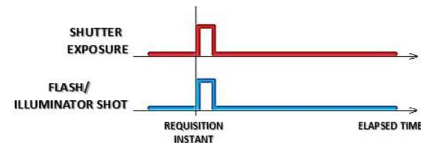
Figure 2 – Comparing diagram of shutter and output flash trigger with flash in Single Mode
