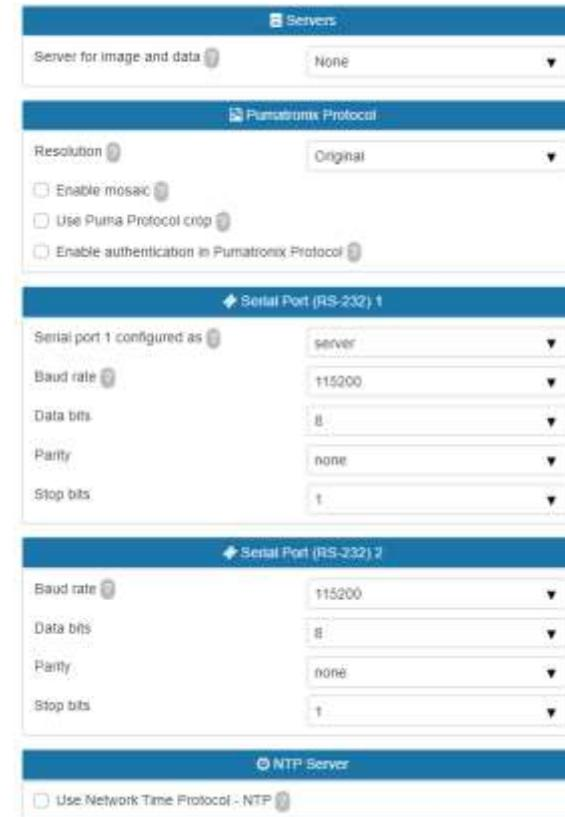
Figure 28 – Servers Settings at ITSCAM Web interface
