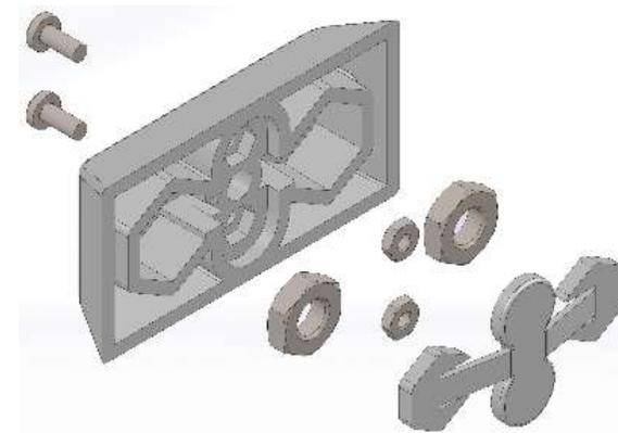
Figure 17 – ITSCAM bracket assembly
