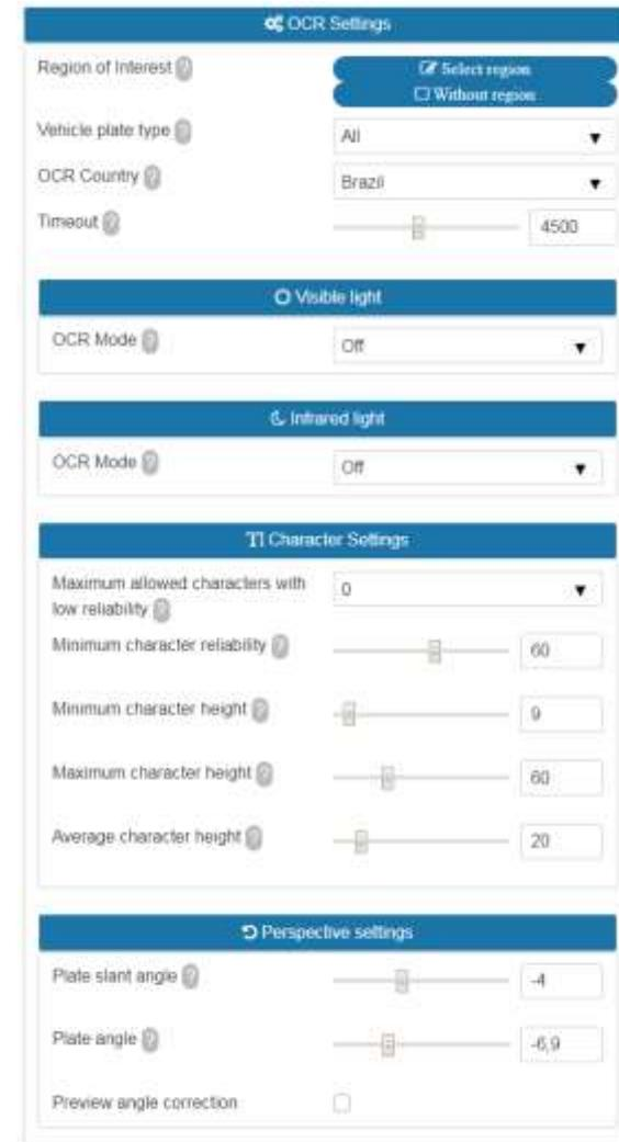
Figure 43 – PART B - OCR Settings at ITSCAM Web interface
