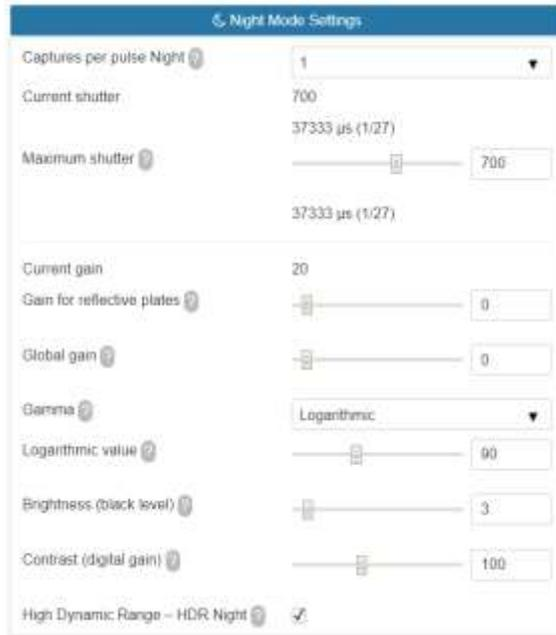
Figure 39 – PART B - Light Settings at ITSCAM Web interface
