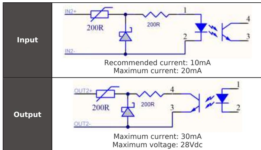
Figure 8 – Isolated input and output circuits
