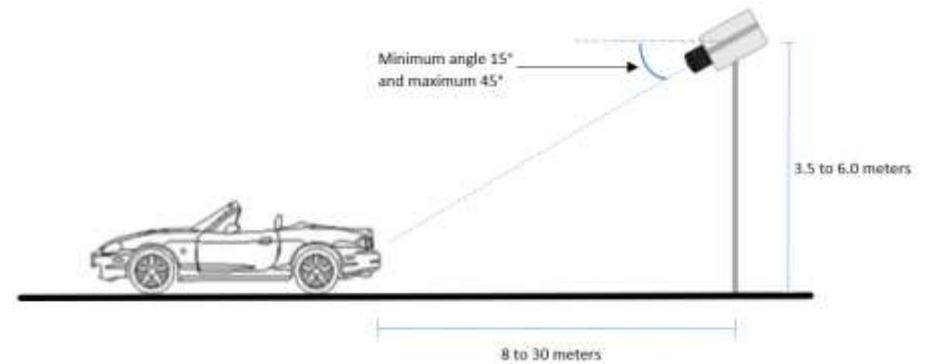
Figure 14 – ITSCAM installation for traffic control (side view)
