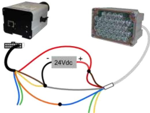
Figure 7 – Connection example of ITSCAM with ITSLUX
