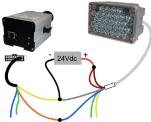
Figure 9 – Connection example of ITSCAM POE with ITSLUX
