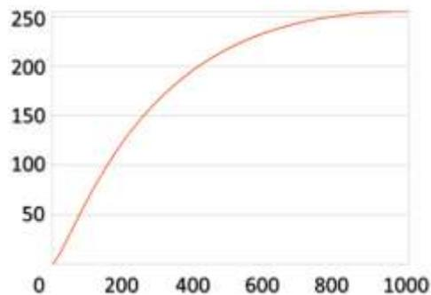
Figure 21 – Example of a gamma curve (Gamma value: 140). It converts sensor pixel value (that varies from 0 to 1023) in a logarithmic way to 8-bit value (that varies from 0 to 255)
