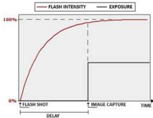
Figure 3 – When light reaches its peak, shutter fires
