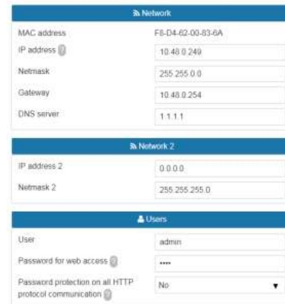
Figure 27 – Network Settings at ITSCAM Web interface
