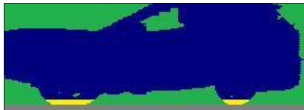
Figure 45 - Magnetic Profile that can identify a car
