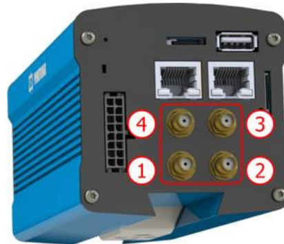
Figure 14 - SMA connectors for the antennas (there may be variations depending on the model*)
