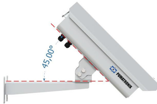
Figure 15 - Maximum Angle of Inclination of the ITSCAM FF 450 Protection Box
