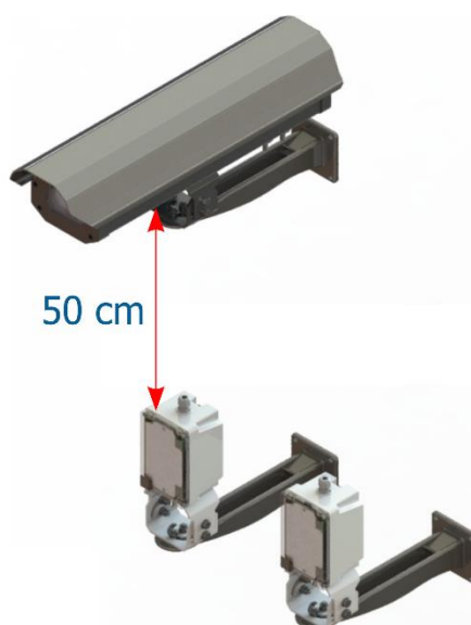
Figure 9 - Example of the application of the illuminator considering the minimum distance in relation to ITSCAM FF 450
