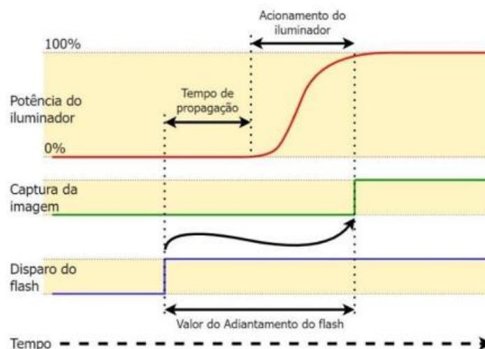
Figure 13 - Moment of Shutter activation after flash intensification
