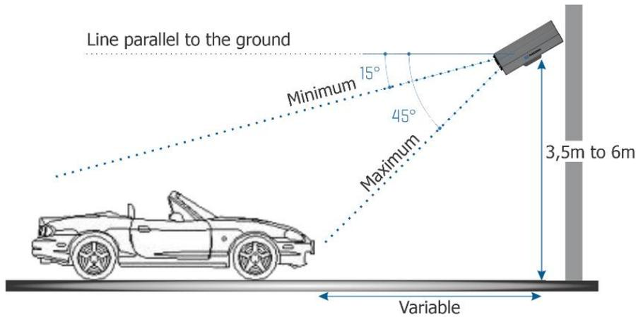
Figure 17 - Side View of the Installation Front Positioning
