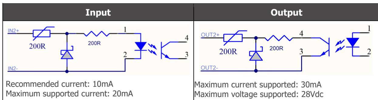
Figure 12 - ITSCAM 400 isolated input/output signal circuit
