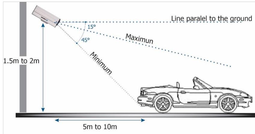
Figure 19 - Side View of the Installation Rear Positioning
