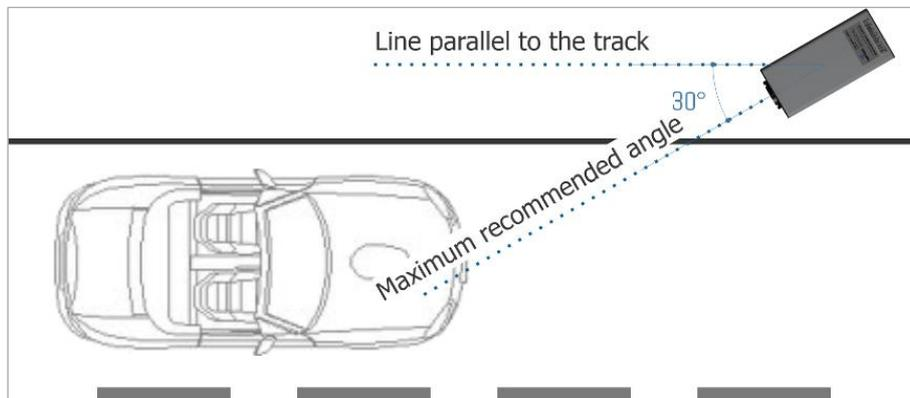
Figure 18 - Top View of the Installation
