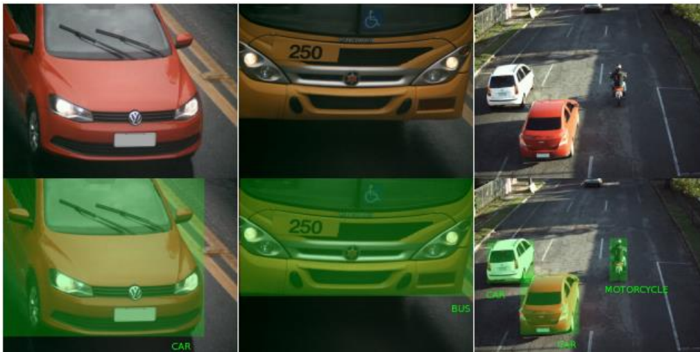
Figure 1 - Classifier application examples: Top: images to be processed by the Classifier; Low: images overlaid with information obtained by the Classifier; Left and center: closed type images; Right: panoramic image
