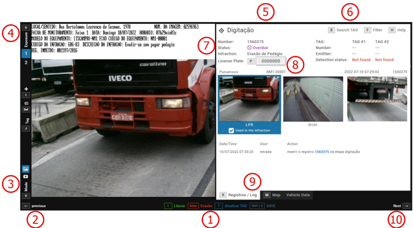
Figure 22 - Screen of a stage of manual Validation: 1) Screening action configured* for the stage, 2) Returns to previous record, 3) View video selection, 4) View of captured images, 5) Screening stage identification, 6) Search TAG filters Options** for searches, 7) Record status, 8) Field for editing the registered plate, 9) View the record data, 10) Proceed to the next record
