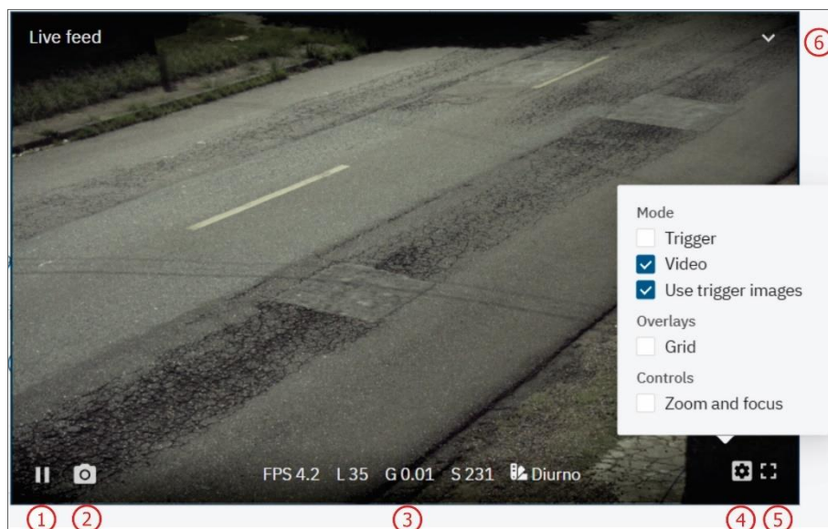
Figure 9 – Pop-up live view window: 1) Pause live view; 2) Take photo; 3) Level of FPS, Gain, Shutter and Photo Profile values active; 4) View settings; 5) Full screen; 6) Minimize window
