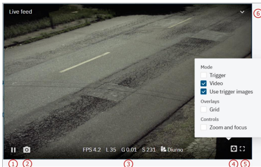
Figure 9 – Pop-up live view window: 1) Pause live view; 2) Take photo; 3) Level, Gain, Shutter and Photo Profile values active; 4) View settings; 5) Full screen; 6) Minimize window
