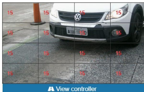
Figure 22 - Importance coefficients (Weights) of the regions demarcated in the image, when accessing Settings > Weights
