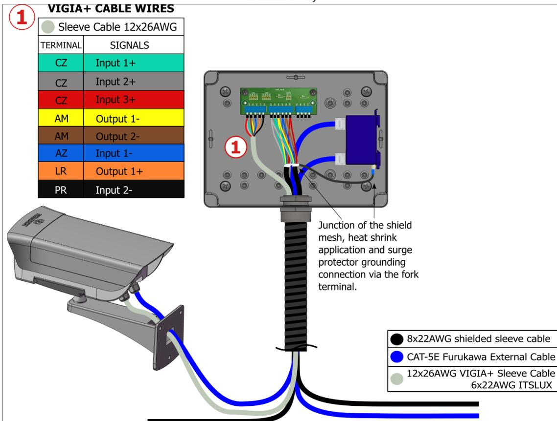
Figure 16 - Connection Diagram for ITSCAM VIGIA+ device on Rear or Panoramic Post (without illuminator)
