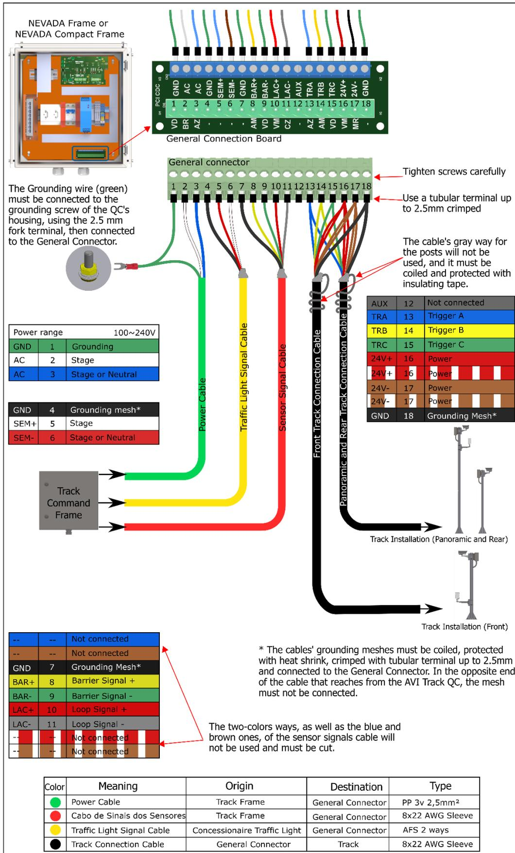
Figure 22 - Connection Diagram with the General Connection Board
