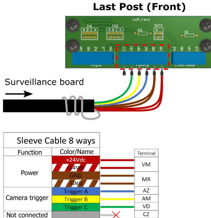
Figure 18 - Wiring Diagram for the 8-Core Sleeve Cable in the Front Catchment Post Junction Box
