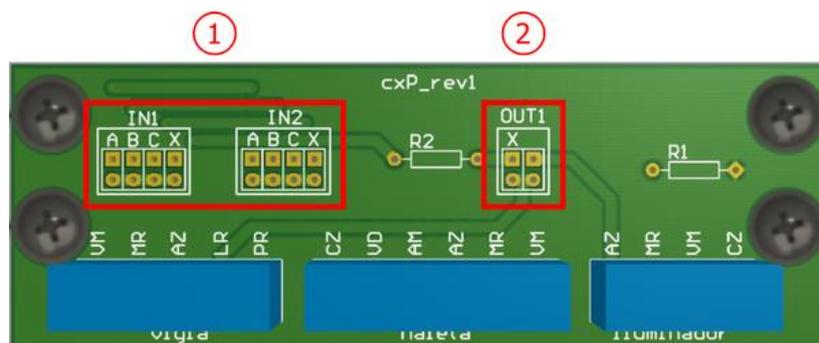
Figure 20 - Connections available on the Terminal Box plate: 1) Input Signals, 2) Output Signal
