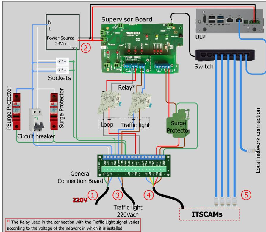
Figure 24 - NEVADA Compact Frame Wiring Diagram
