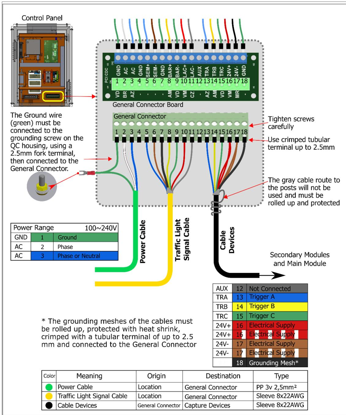
Figure 10 – Tertiary Module General Connector Diagram
