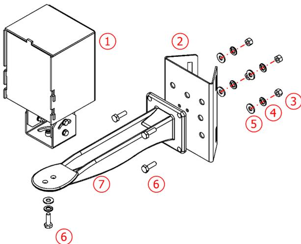
Figure 6 - ITSLUX Illuminator Cage Bracket Parts
