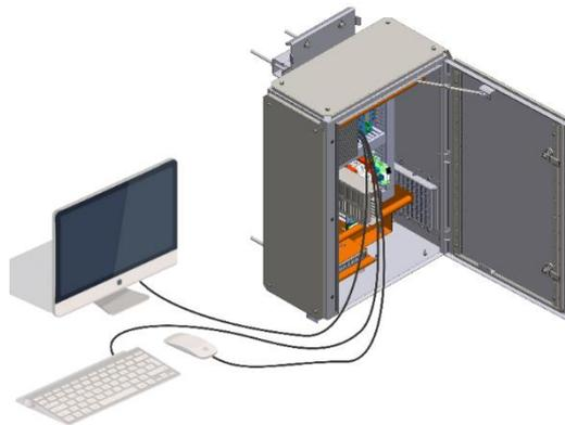
Figure 1 - Access to the ULP to set up the network type
