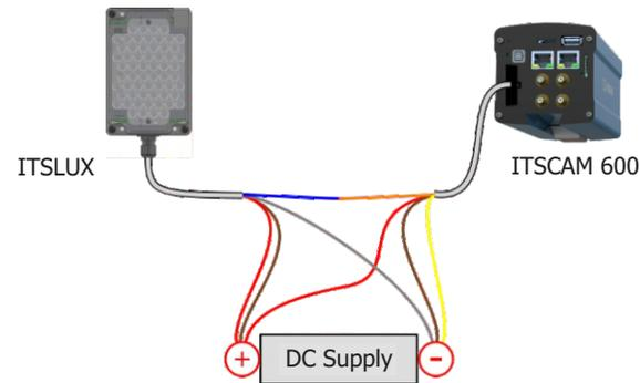
**20.** Protect connections with splice connectors or similar structures.
