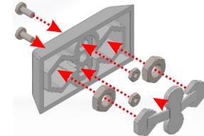
4. Insert the Fastener into the rail located at the top of the illuminator housing, keeping the screws loose or open enough for the assembly to slide onto the rail:
