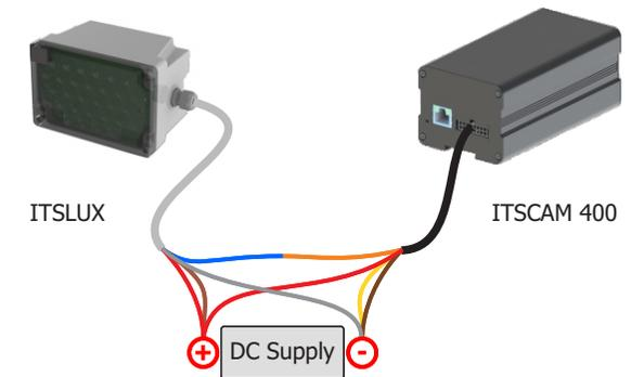
**30.** Protect connections with splice connectors or similar structures.
