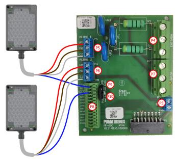
**31.** Check if jumper P9 and P10 are closed when connecting to IO+ of Illuminators 1 and 2.
