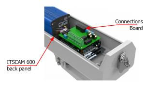
4. Use the connectors available on the back panel of the ITSCAM 600 device:
