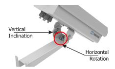
**41.** Tilt the equipment on the base until the best framing fit, considering the maximum angle limit of **45°** for vertical tilt. Greater angles of vertical inclination generate significant deformations in the generated images.
