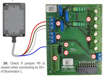
**30.** Connect the wires of the 2 ITSLUX cables to the P5, P6 and P8 connectors, following the colors indicated on the *Connections Board*:
