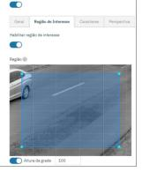
**38.** Enable the Grid Height display with a value of 25 for fine-tuning Zoom and Focus. The license plate characters are at the ideal reading size when they fit within this height.
