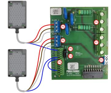
19. Check that jumpers P9 are closed when connecting to Io1+ of Illuminator 1.
