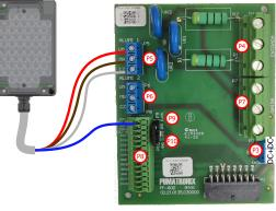
17. Check that jumpers P9 are closed when connecting to Io1+ of Illuminator 1.
