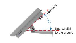
**29.** Tilt the equipment on the support until the frame is best adjusted, considering the maximum angle limit of 45° for vertical inclination. Higher angles of vertical inclination generate significant deformations in the images.
