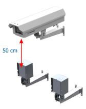
When using an Illuminator in conjunction with the ITSCAM FF 450, check the product specifications to determine the minimum and maximum distance that must be observed in relation to the position of the object to be illuminated.
