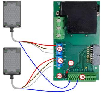
**19.** Check that jumpers P9 and P10 are closed when connecting to Io1+ and Io3+ of Illuminators 1 and 2.
