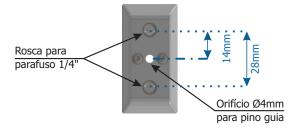
**24.** Reassemble the Fixing Mechanism following the sequence indicated in the image, if it detaches from the housing of ITSCAM 600:
