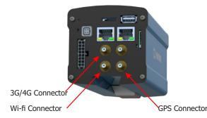
5. Connect the available antennas to the respective SMA connectors named 3G/4G, Wi-Fi and GPS.
