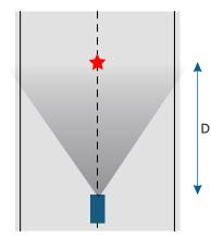
**22.** Secure ITSCAM 600 considering the minimum height limits specified for the location. The linear distance **D** from the vehicles' crossing point varies according to the estimated range of the lens model. Refer to the Product Manual for more information.
