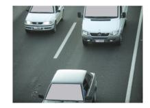
**33.** Use the *Autofocus* function when the ITSCAM 600 model has motorized lenses or adjust *Zoom* and *Focus* by accessing the *Image* > *Profiles* menu at *Lens* tab, until the characters become clear in the image viewed.
