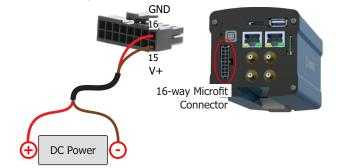
This equipment must be supplied with a direct current (DC) source with a voltage of 12 VDC or 24 VDC. Do not connect any of the inputs directly to the mains (AC)!
