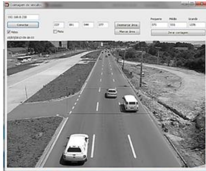
Figure 5 - ITSCAM VIGIA+ Vehicle Counter Interface
