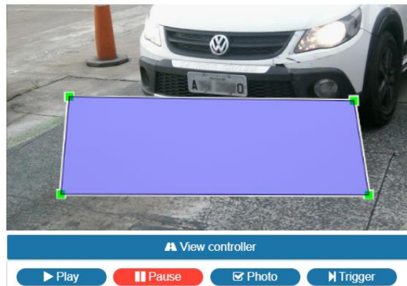
Figure 26 - Image Preview with a region of interest (ROI) configured for OCR, which searches for plates inside the rectangle
